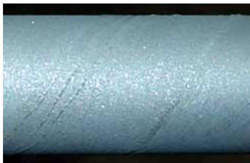
Figure 1. Thin Layer of Wet Lubricant Compound on Shaft Surface
