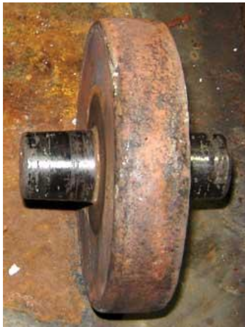
Figure 5. Glazed Axle Surface
