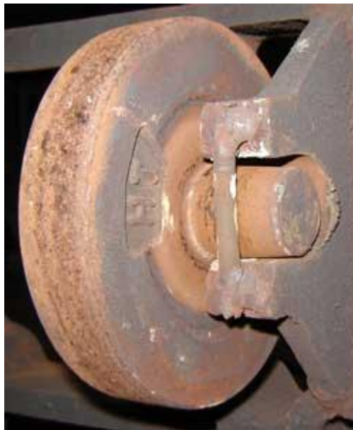
Figure 4. Graphite Grease-lubricated Surface of Wheel After Exiting Furnace
