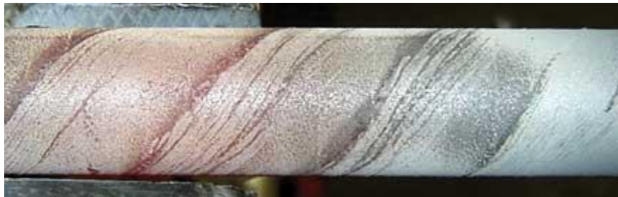
Figure 2. Dry, Powdery Lubricant Film After Heating
