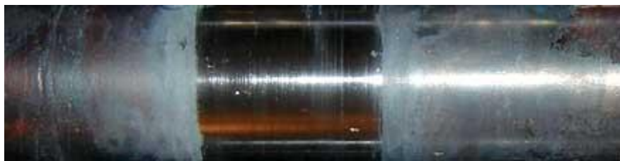
Figure 3. Glaze Formed by Solid-film Lubricant
